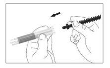
3. Insert the plunger rod (DPM) in the syringe barrel to eliminate air and press the solder paste.
