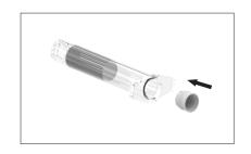
2. Place the piston into the syringe barrel.
