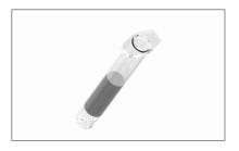
1. Fill in the syringe barrel with solder paste.
