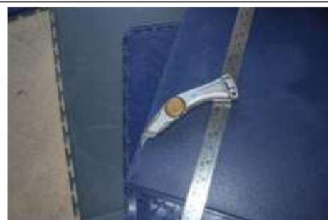
Stanley knife with concave blade
